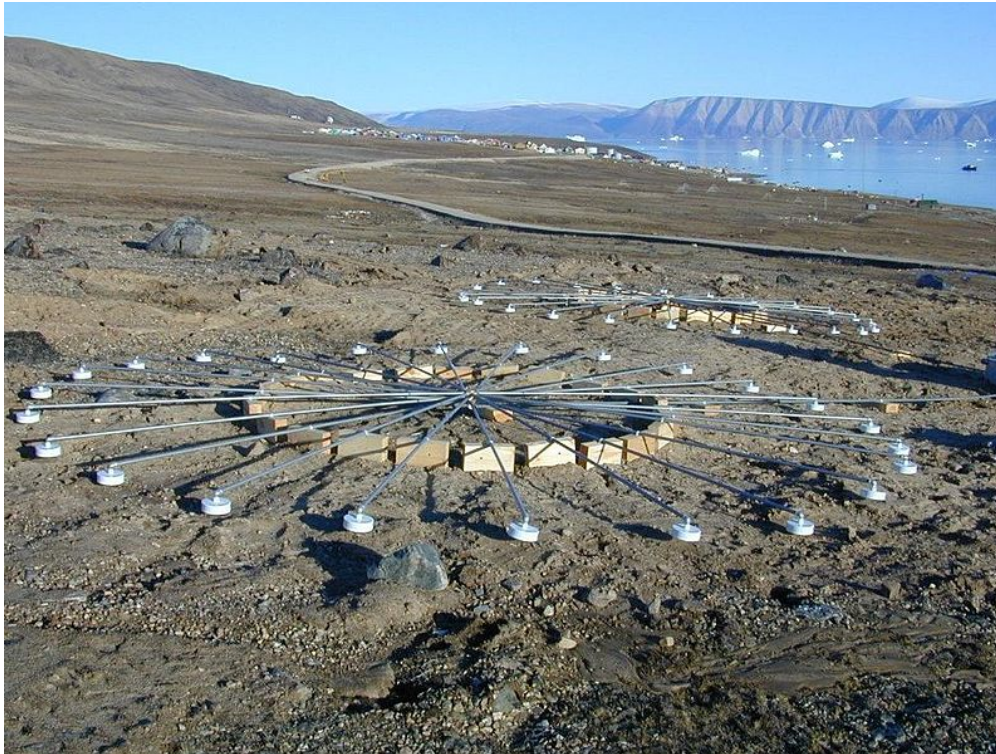
Figure 1: CTBTO Infrasound 'Pipe Array' - Greenland [3]
