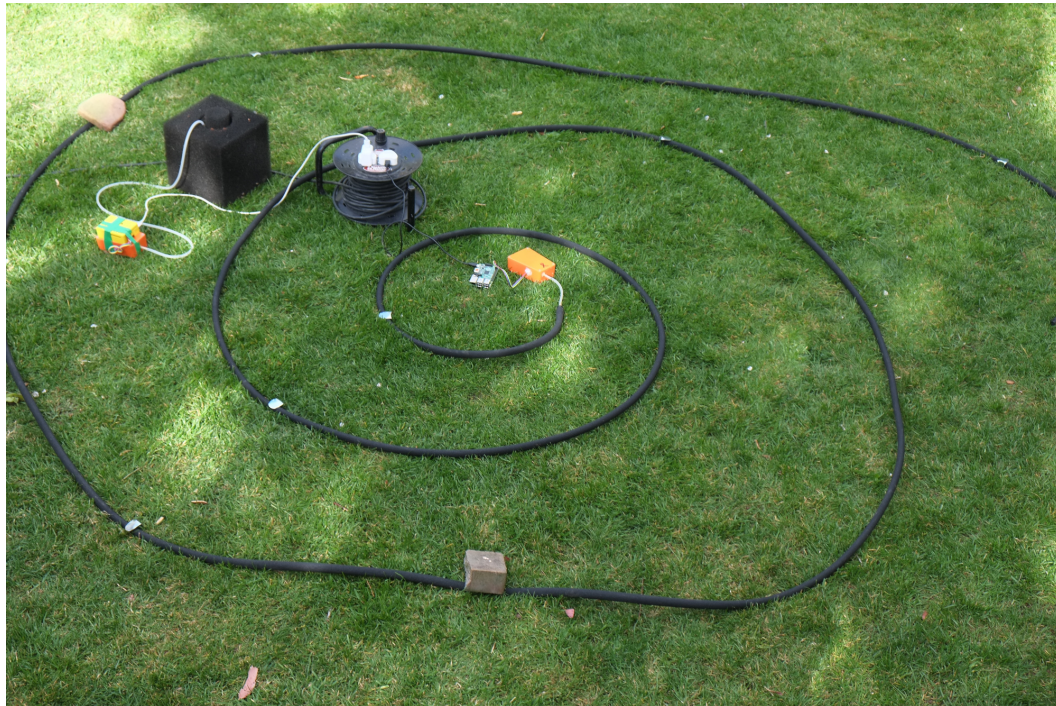
Figure 6: Pond filter tested alongside spiral hose
